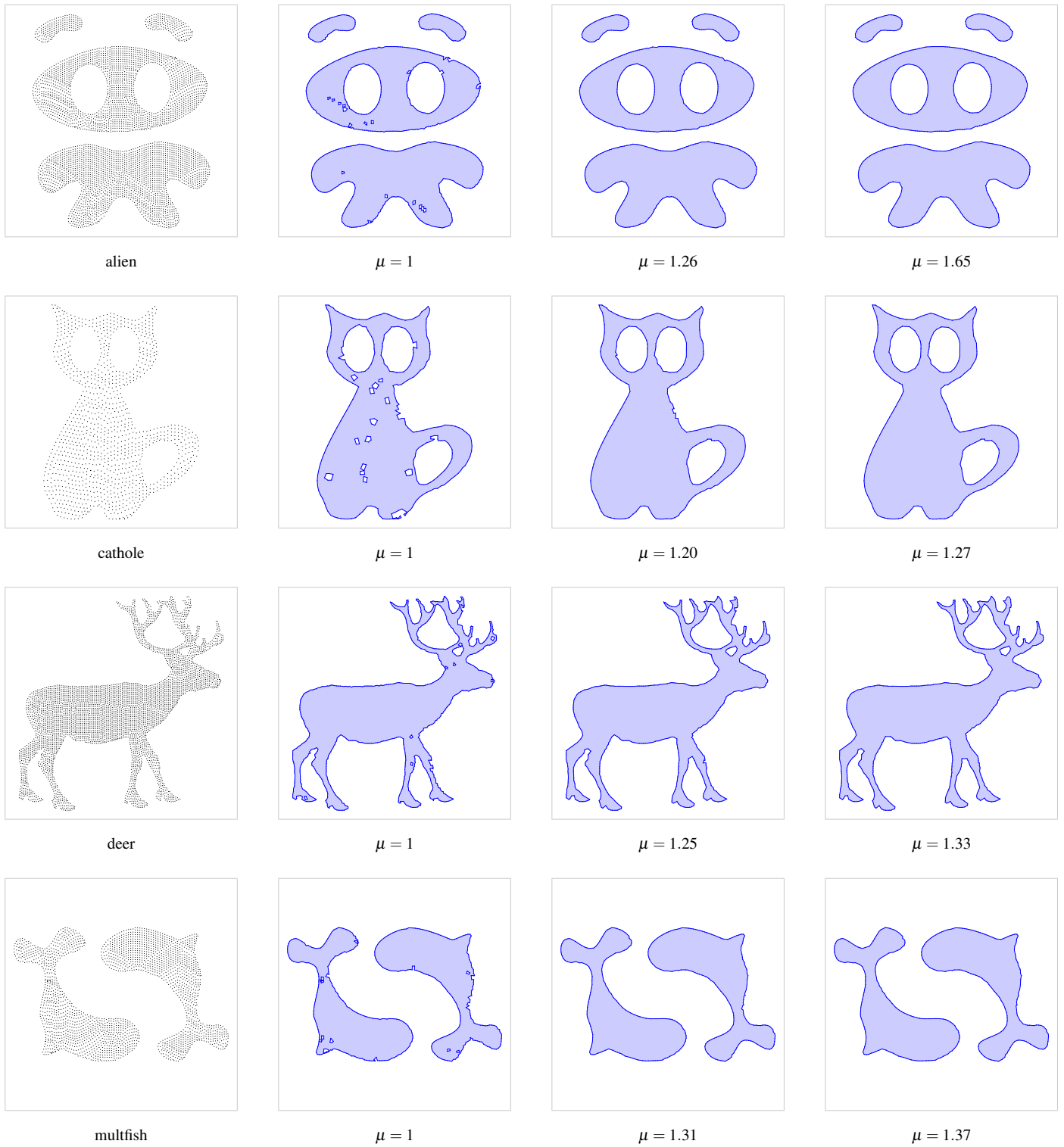
Fig. 13. First \mu that recovers topology (third column); next \mu that gives smooth reconstruction (fourth column).
