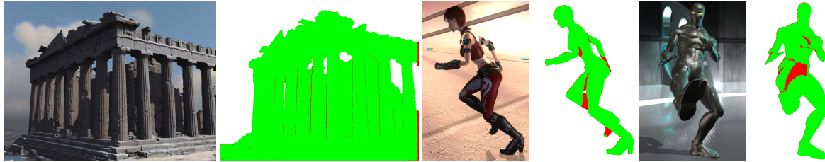
Figure 1: Real-time rendering applications exhibit a considerable amount of spatio-temporal coherence. This is true for camera motion, as in the Parthenon sequence (left), as well as animated scenes such as the Heroine (middle) and Ninja (right) sequences. Diagrams to the right of each rendering show disoccluded points in red, in contrast to points that were visible in the previous frame, which are shown in green (i.e., green points are available for reuse). [Images courtesy of Advanced Micro Devices, Inc.]
