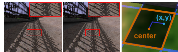
Figure 15: Light-space perspective shadow mapping [WSP04] (left) gives good results for a shadow map resolution of 1024^2 and a view port of 1680 \times 1050 , but temporal reprojection (middle) can still give superior results because it uses shadow test confidence, defined by the maximum norm of shadow map texel center and current pixel (right).
