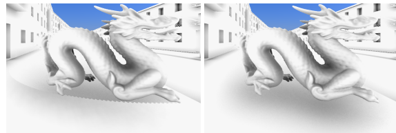
Figure 22: Moving dragon model using no invalidation (left, causing severe artifacts in the shadow), and using an invalidation factor set to a proper value (right, no artifacts).
