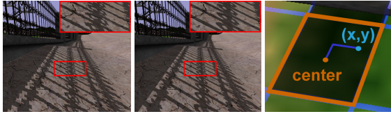
Figure 14: LiSPSM (left) gives good results for a shadow map resolution of 1024^2 and a view port of 1680 \times 1050 , but temporal reprojection (middle) can still give superior results because it uses shadow test confidence, defined by the maximum norm of shadow map texel center and current pixel (right).
