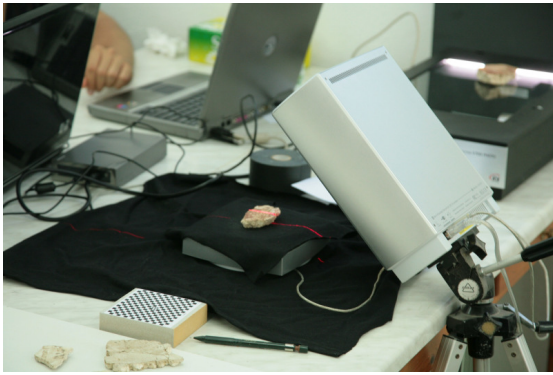
Figure 3: Using an off-the-shelf 3-D scanner (front), positioned at a 45-degree angle relative to a motorized turntable, we can acquire the front, back, and sides of a fragment with a single manual flip. A 2-D scanner (rear) simultaneously acquires high-resolution color and normals.
