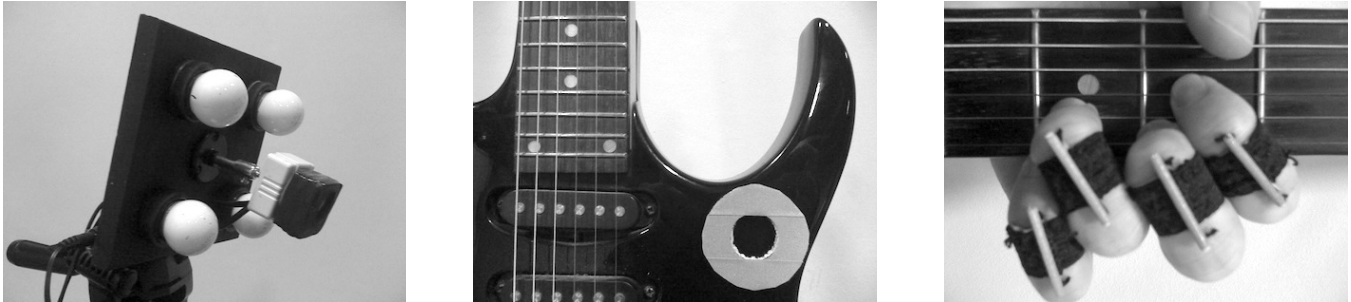
Figure 1: Capture hardware. On the left, an infrared camera surrounded by four infrared light sources. In the center, a hollow disk made with reflexive material. Four of them are used to locate the plane containing the ROI. On the right, middle-phalanges gloves with small rods coated so as to easily reflect light.
