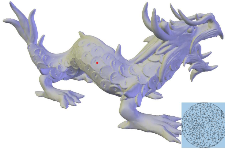
Figure 1.5: Example of a mesh processing technique shown on the Asian Dragon from XYZ RGB Inc. The surface around the selected vertex (in red) is parameterized in two dimensions and shown in the bottom-right corner.
