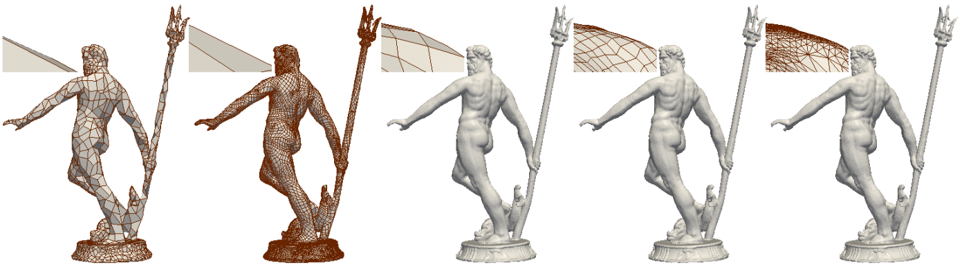
Figure 12: The Neptune model simplified and tiled to its base mesh (left), increasing the resolution to level-3 (second from the left), level-6 (third) and level-9 (fourth); and the original dense mesh (right). Each upper-left corner details the top of the model’s head. Quads drawn are in fact triquads.
